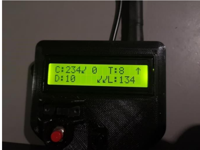
Figure 12: LCD handheld receiver with backlight and custom 3D printed enclosure. (Source: Jacob Larsen)
