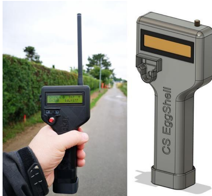
Figure 15: Updated ruggedized custom enclosure for the LCD handheld receiver. (Source: Jacob Larsen)
