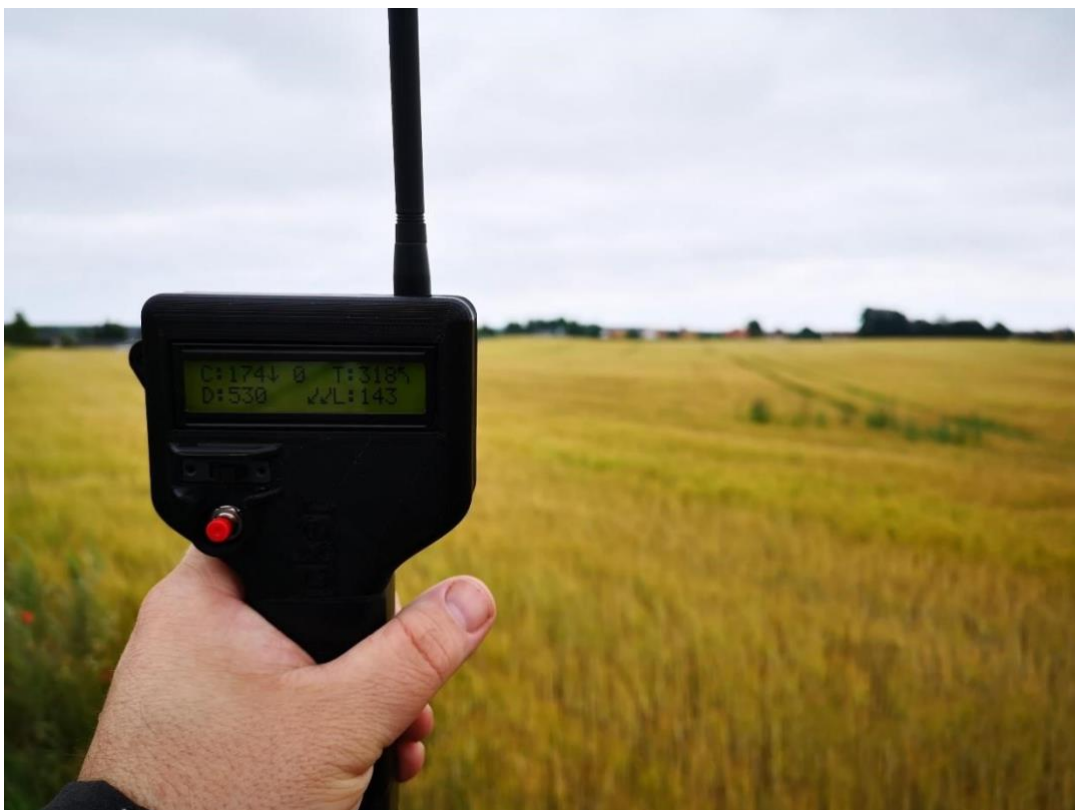
Figure 10: LCD handheld receiver detects GPS transmitter at a distance of 530 meters. (custom enclosure, 3dB stub antenna, SMA board connector options) (Source: Jacob Larsen)
