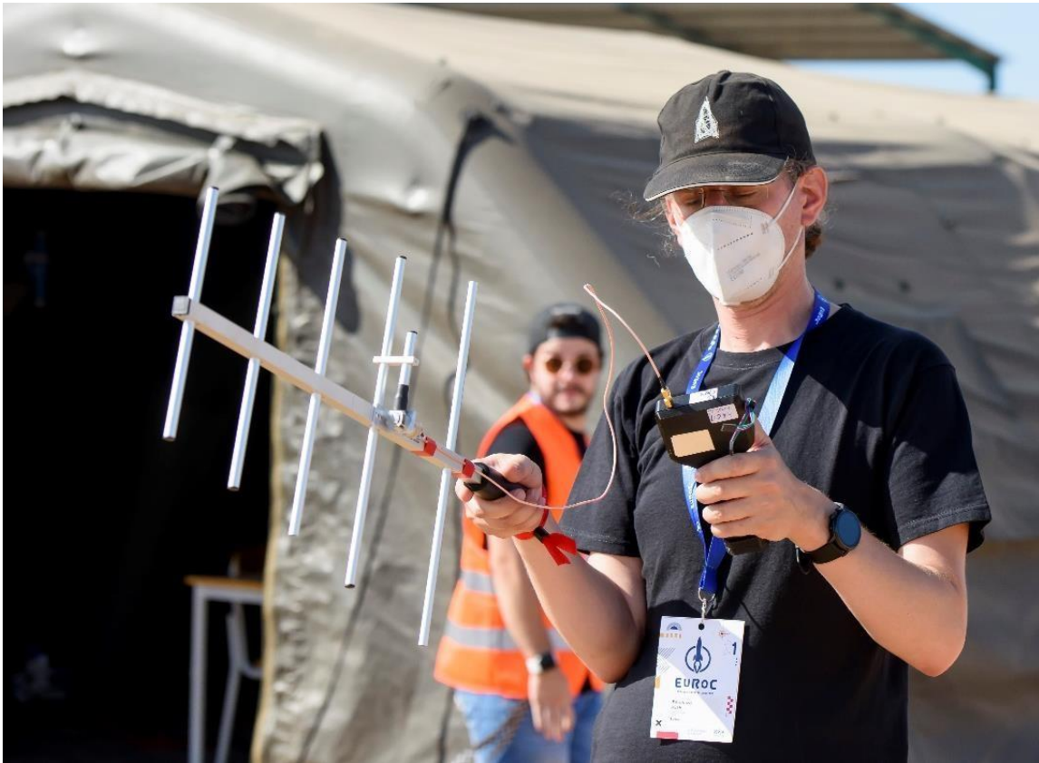
Figure 14: Yagi 5-element high gain antenna.
