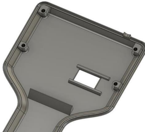
Figure 19: Rear section illustrating the programming port opening and where to tap M3 threading. (Source: Jacob Larsen)
