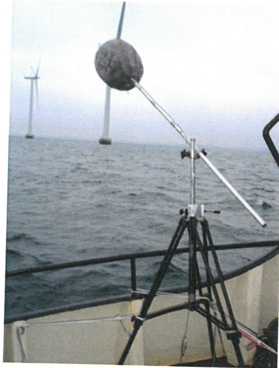
Figure 1 Mounting of microphone on board the vessel. The microphone is supplied with an extra wind shield.
